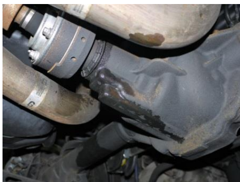
8.8 pinion seal leak
