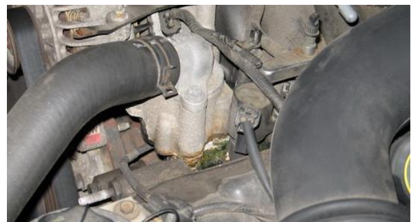
Seeping thermostat housing on a 4.6L. This is a cooling system compromise. Fix it.
